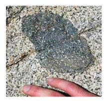
d. **Surface Chipping**: Different stones have different mineral compositions. Stones that contain softer or flaky minerals, such as mica, will often have spots on the surface or the edge that flake away. There is no process to eliminate this chipping and should be considered when choosing a stone with these characteristics.
